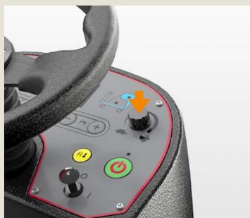
Adjust the maximum speed with the speed adjustment dial.
