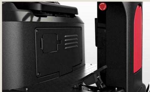
Connect the battery charger to the charging inlet on the machine and switch on the charger.
