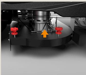
To install the brush/pad holder, pull up the metal handle and slide in the brush/pad holder until it stops against the pins in the proper position and release the handle. Put back the side skirt
