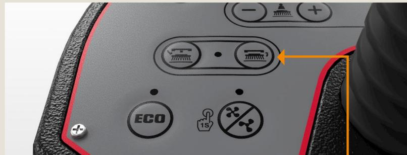
Turn the main key to on and press the click on button to install the brush automatically. Deck will lower and brushes turn slowly to attach.
