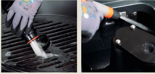
Empty the tank with the hose in the back. Empty and clean the debris tray in the tank, flush&clean out the recovery tank.
