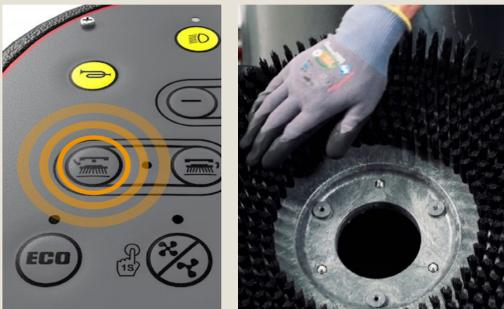
With the key turned on press the brush click off button to remove the brushes/pad holders for inspection and cleaning.
