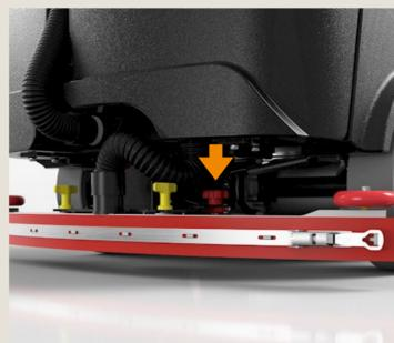
Adjust squeegee angle and blade pressure for optimal water pick-up by turning the adjustment knob on the support.
