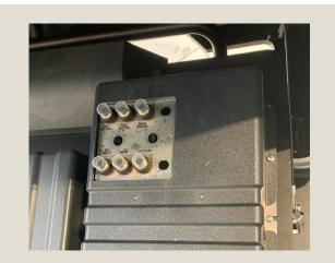
5. Check the vacuum and filter shaker circuit breakers.
