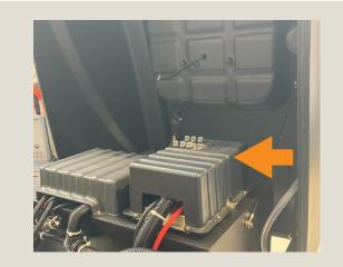
3. Open the machine cover and check the broom circuit breakers.
