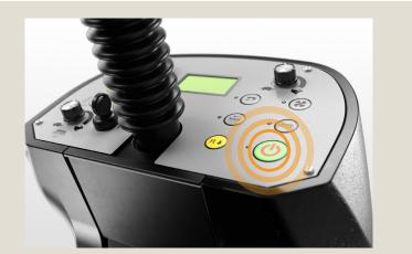
Press the OneTouch<sup>™</sup> button to enable all sweeping functions, the brooms will lower automatically.
