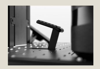
Press the front flap pedal to open the front flap for sweeping larger debris.
