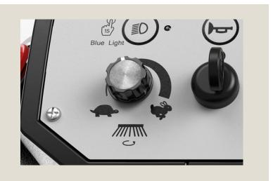
Adjust the speed of the side brooms by changing the side broom speed knob.
