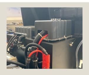
3. Check if the main battery connector is properly connected.
