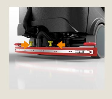
Install the squeegee and fix it by using the two knobs.
