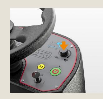
Adjust the maximum speed with the speed adjustment dial.
