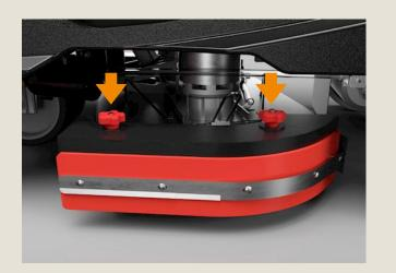
Loosen the two knobs to remove the side skirt.
