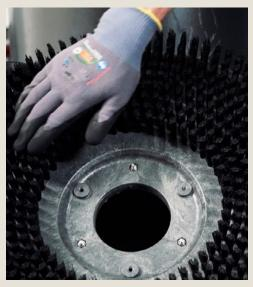
With the key turned on press the brush click off button to remove the brushes/pad holders for inspection and cleaning.
