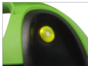
WARNING LIGHT FOR SPEED CONTROL >20 M/S
